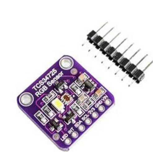
Figure 3. TCS34725 RGB Color Sensor module with integrated IR blocking filter.
