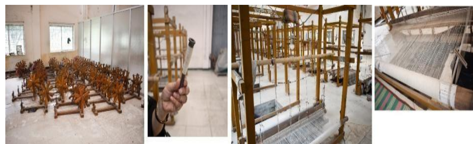
Fig. 31. (From left) Image (a), (b), (c), (d) parallelly showing customized hand spinning wheels, Natai or warping the yarn, the customized Muslin weaving frame, the closer view of Muslin fabric warped in the waving frame in 'Dhakai Muslin House' (Source: Author)
