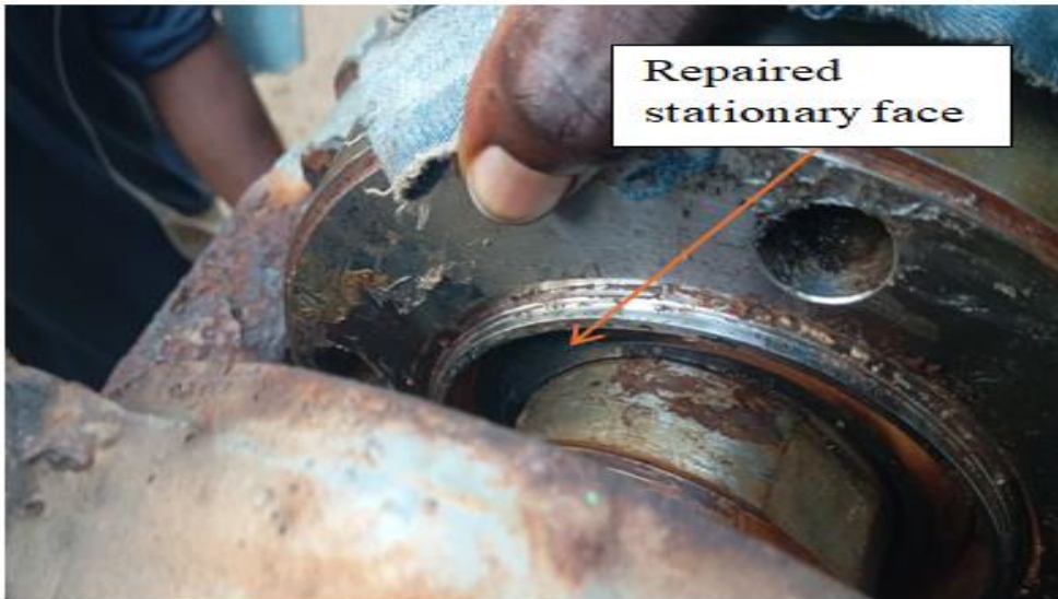
Fig 7. Repaired the stationary mechanical seal face
