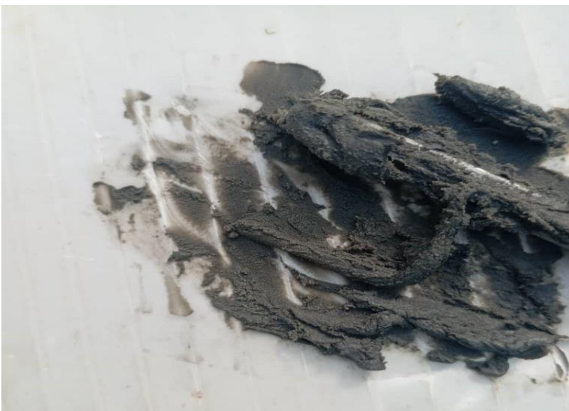
Fig 6. Mixing of epoxy composite material
