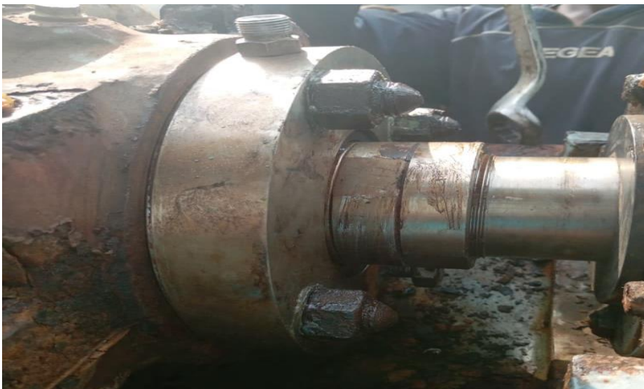
Fig 8. Boxing up of the mechanical seal face
