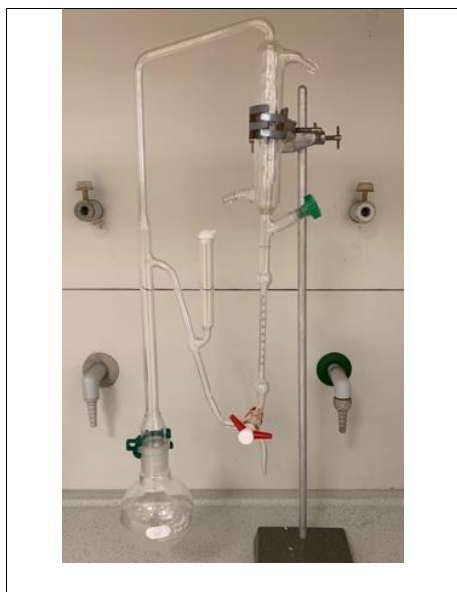
Figure 5: The steam distillation apparatus, where the steam is generated in situ (in existing flask). It is a combination of a glass condenser and a flask for continuous removal of the water, that is produced during reflux. Four grams of dried Callistemon samples could be added with 100 mL of distilled water in a 250 mL round-bottom flask.
