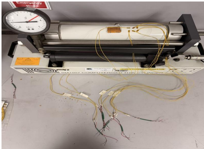
Figure 2: 2003 SM1007 Thin Cylinder Apparatus with installed new strain gauges.
