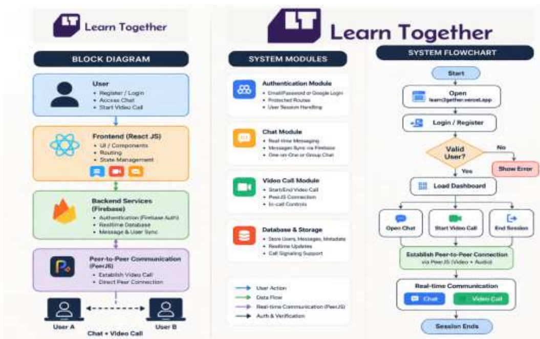
Figure 2. Learn Together System Block Diagram and System Flowchart of User Interaction
