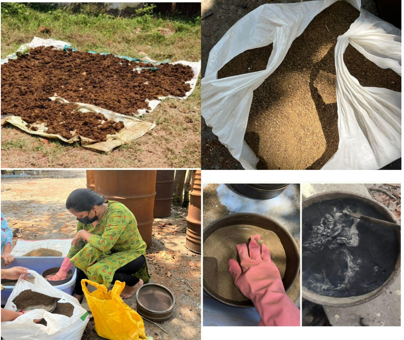
Figure1: Preparation of Cow Dung Ash
