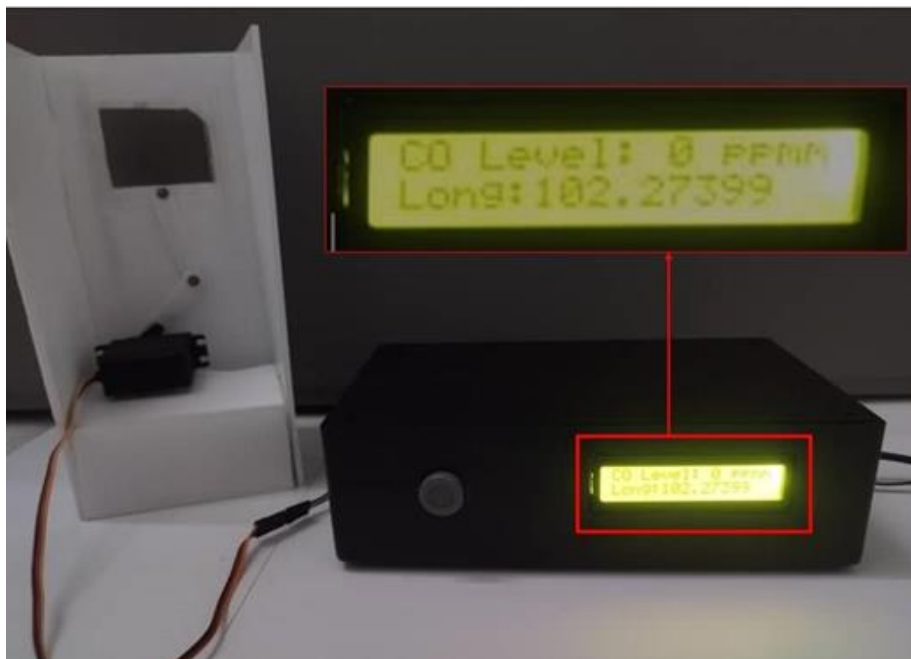
Figure 2. Setup of the Integrated System Prototype (0 ppm – Clean Air)
