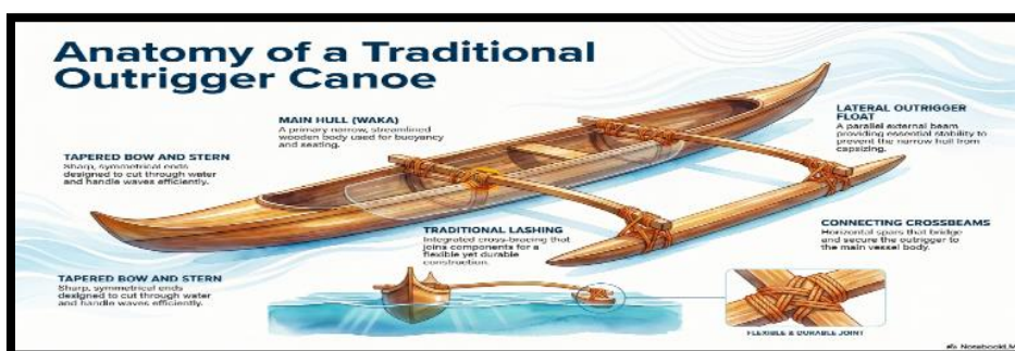
Figure 4: Anatomy of a Single-Outrigger Canoe
