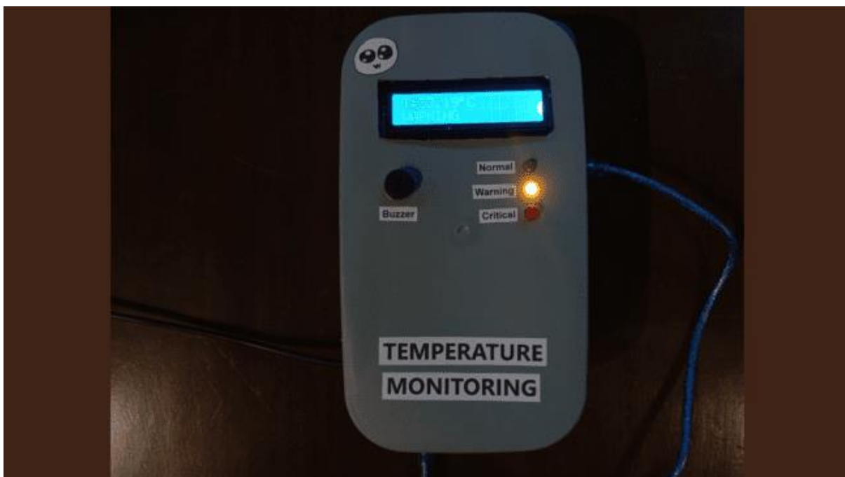
Figure 9. System Result During Warning Temperature Condition
