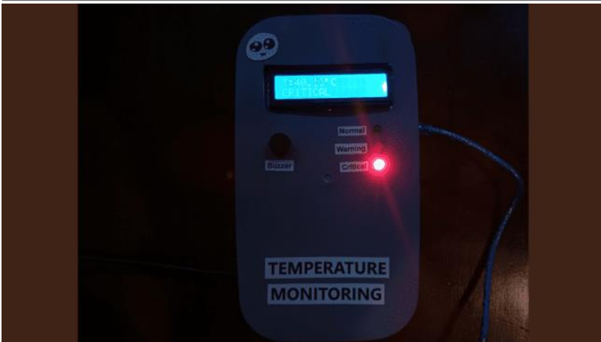
Figure 10. System Result During Critical Temperature Condition
