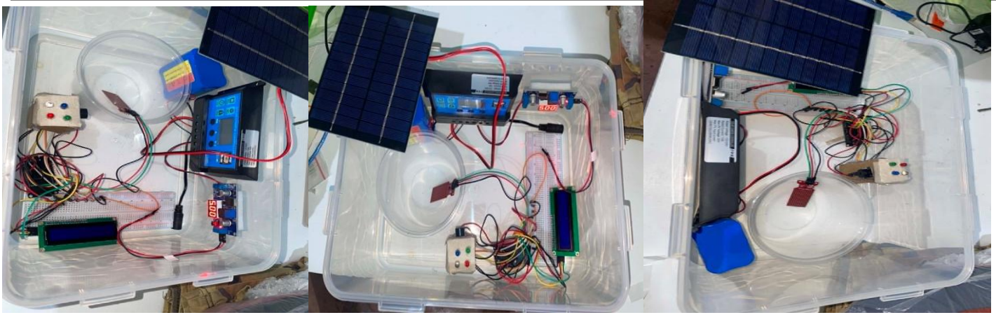
Figure 3. Actual Product of the Solar-Powered Water Level Detection System with Real-Time Flood Alerts and Emergency Light Pole
