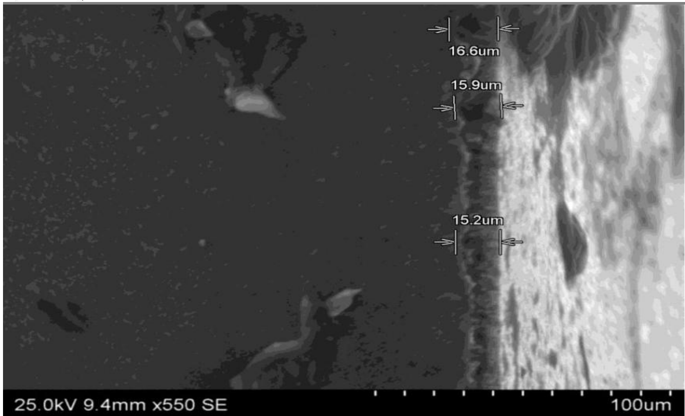
Fig 5.5. SEM image of tool wear using nano coolant for Exp. 14.
