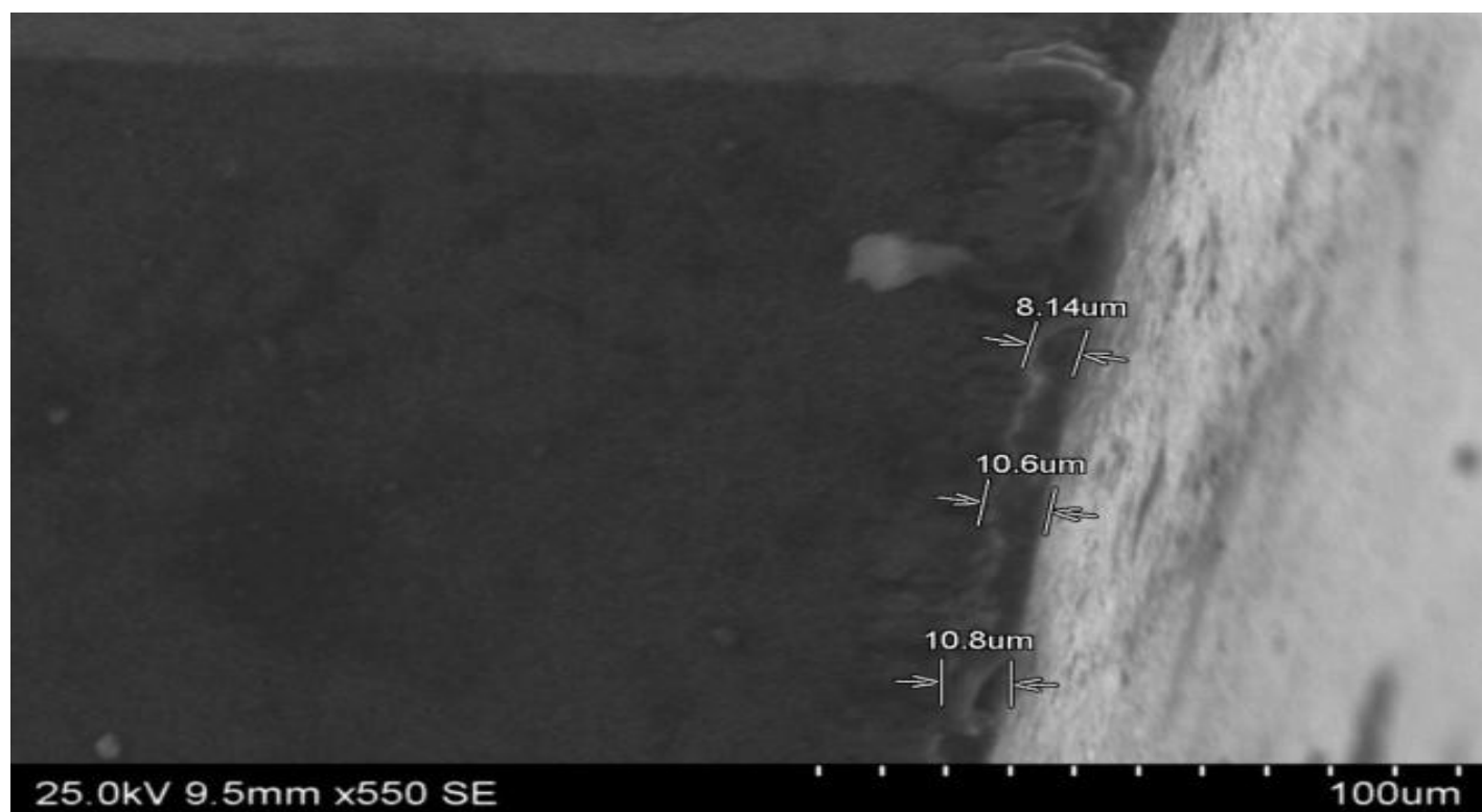
Fig 5.3. SEM image of tool wear using nano coolant for Exp. 1.
