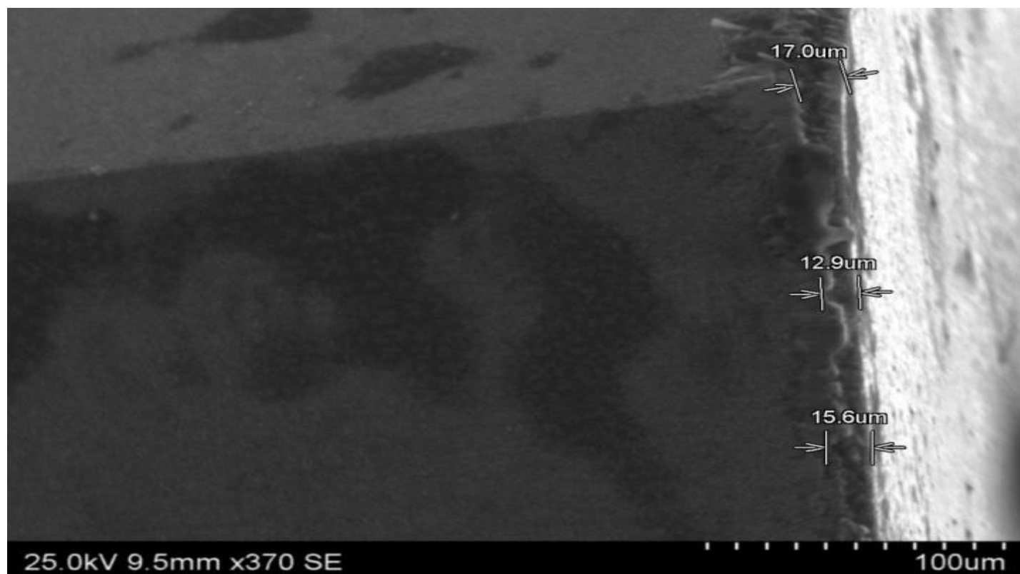
Fig 5.4. SEM image of tool wear using conventional coolant for Exp. 1.
