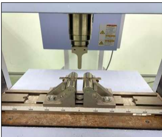
Figure 4: Three-point flexural-test setup
