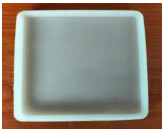
Figure 2: Mould used for impact specimens
