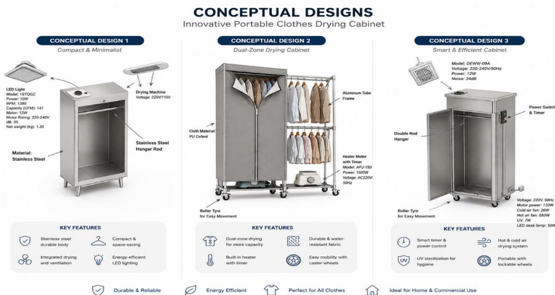
Figure 2. Comparison of three conceptual designs for the proposed portable clothes drying cabinet. Concept 1 features a compact stainless-steel cabinet with an integrated drying unit and LED lighting. Concept 2 adopts a dual-zone drying configuration with a fabric enclosure, aluminium frame, heater, and castor wheels to maximize drying capacity and portability. Concept 3 incorporates a stainless-steel cabinet with a double-rod hanger, timer-controlled heating system, UV sterilization, and mobility features, providing an enhanced solution for efficient, hygienic, and user-friendly clothes drying.
