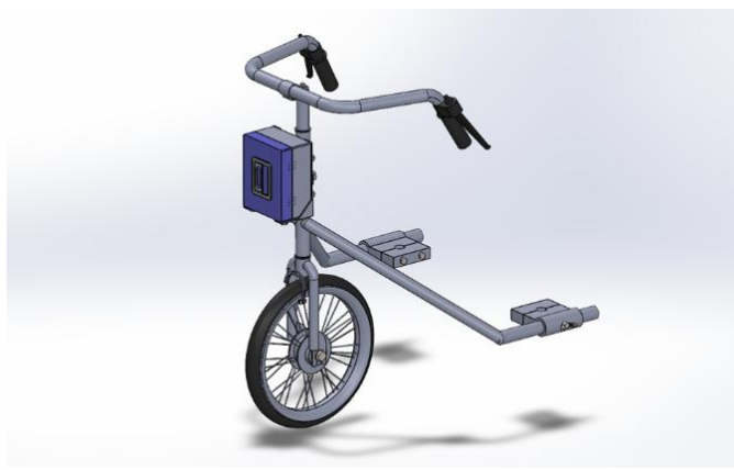
Figure 2: Assembly Drawing of the current Design Handcycle
