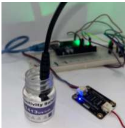
Figure 2. TDS DF robot probe in standard electrical conductivity solution
