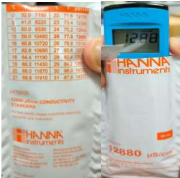
Figure 3. EC Hanna meter in standard calibration solution
