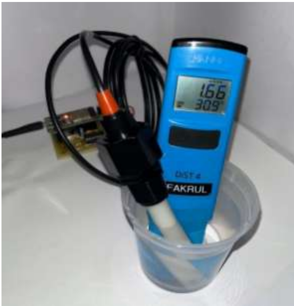
Figure 9. The designed circuit together with EC meter
