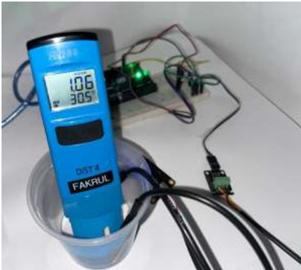
Figure 4. TDS DF robot and temperature with Arduino Uno Proposed circuit design
