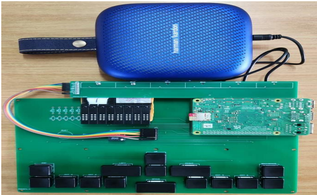
Figure 1: Completed Raspberry Pi-based Braille notetaker prototype.
