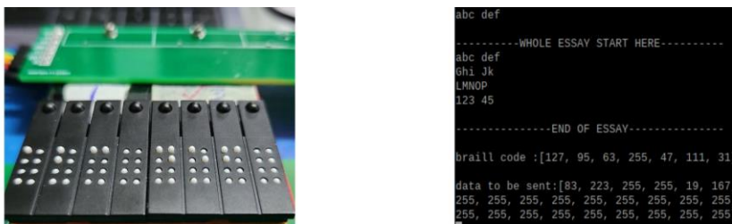
Figure 3: Representative lower-case output on the Braille cells and Raspberry Pi terminal.
