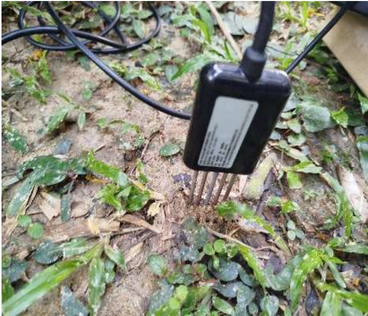
Fig. 3. In-situ field soil testing setup and 7-in-1 Modbus RS485 probe deployment protocol at FTMK UTeM test sites.
