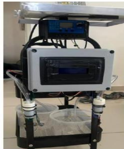
Figure 3. Completed prototype of the solar-powered smart agriculture monitoring and automation system.
