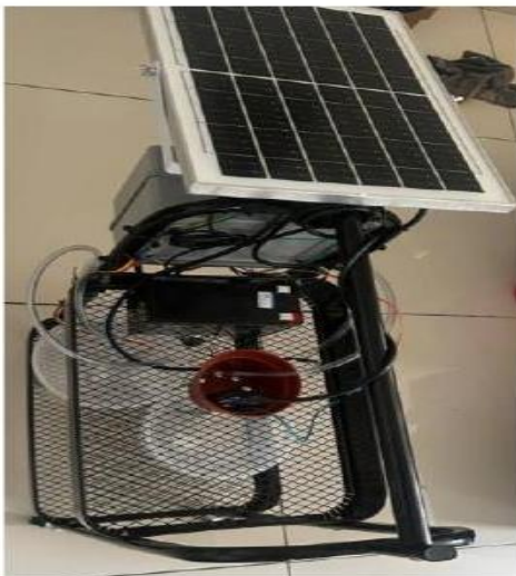
Figure 3. Completed prototype of the solar-powered smart agriculture monitoring and automation system.
