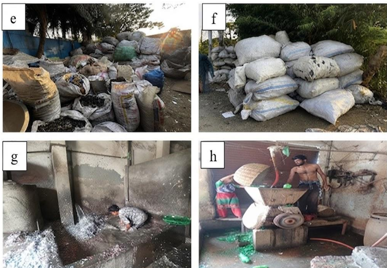
Figure 4. (e) Sorted waste in waste factory, (f) Packaging after recycling, (g) Washing, (h) Cutting.
