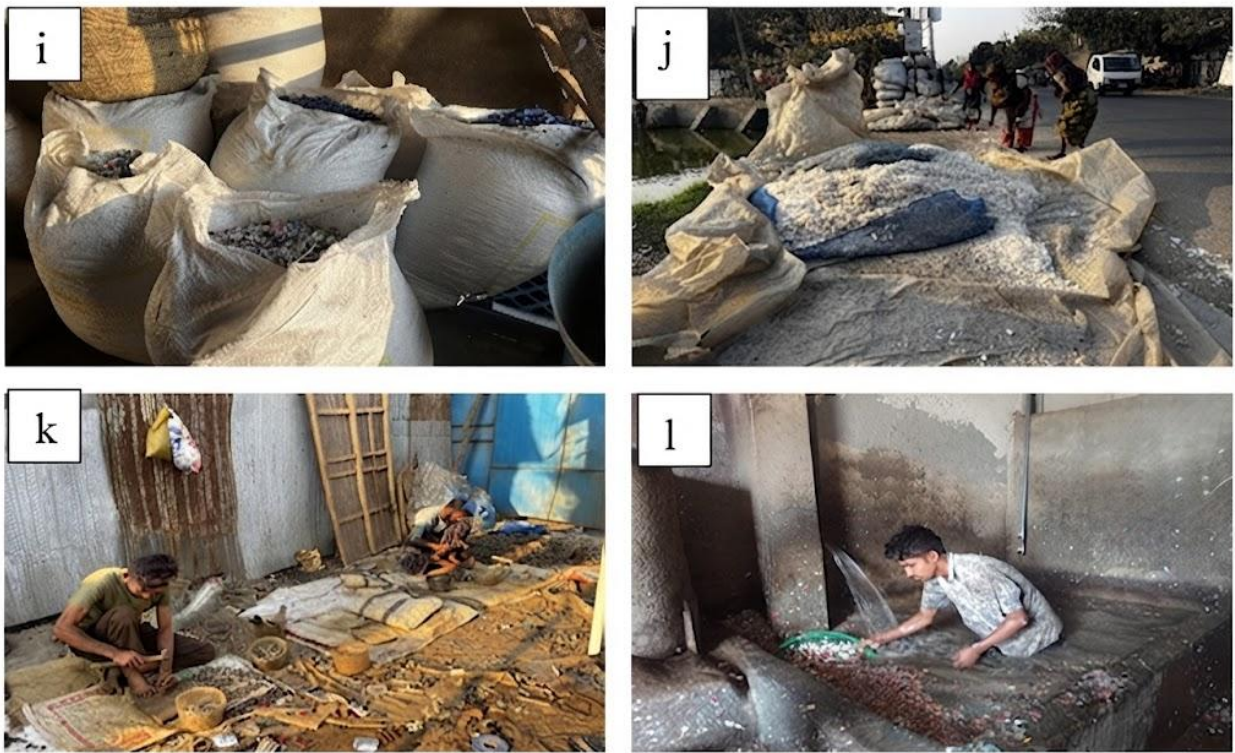
Figure 4. (i) Packing after drying, (j) Drying, (k) Sorting in factory, (l) Separating unwanted things after washing.
