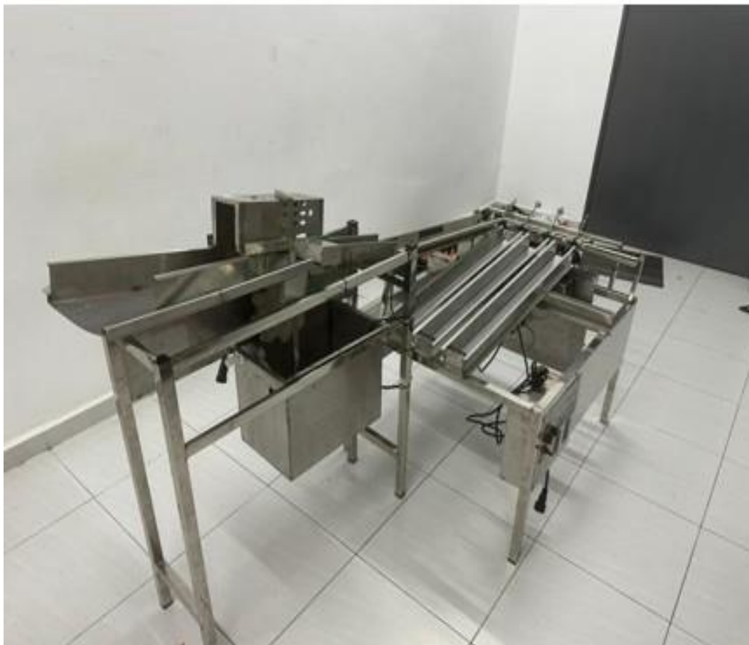
Figure 1. Fabricated semi-automated egg cleaning and sorting system (angled view).
