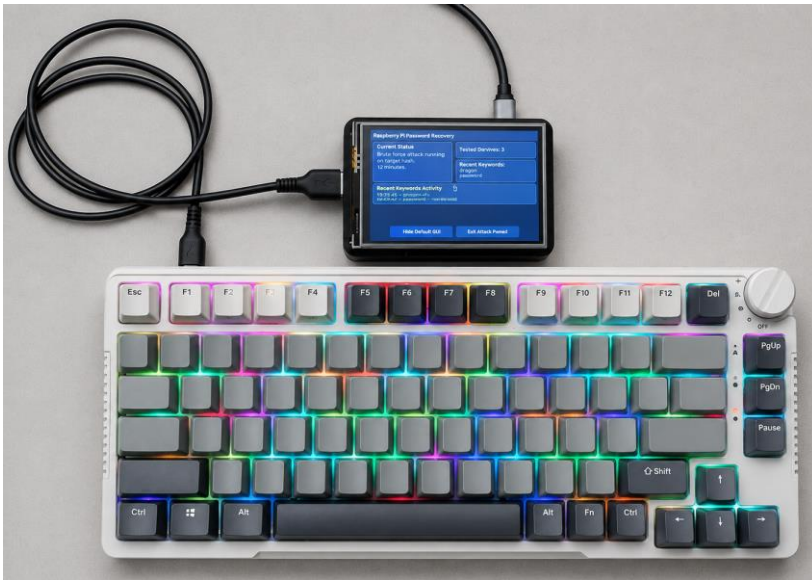
Figure 3.4: Normal-use test configuration with the Raspberry Pi 4 positioned between the keyboard and host computer
