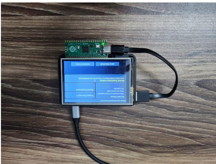
Figure 3.5: Offensive test configuration using a Raspberry Pi Pico as the malicious HID
