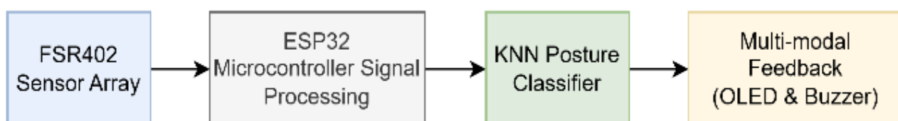
Fig. 1 System block diagram of the smart chair posture detection.
