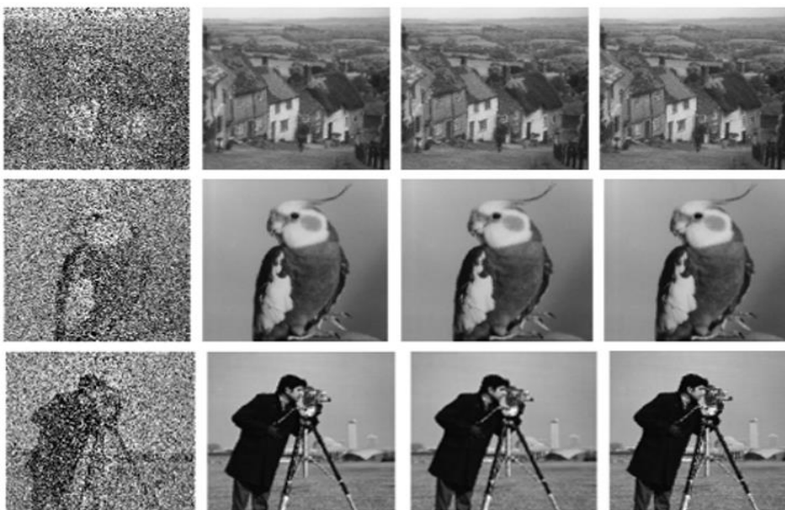
Figure 3. Restoration of Goldhill, Bird, and Camera. From left to right: the images are degraded with 50% salt-and-pepper noise and restored by the MMR (middle), NHMR, and SFA methods, visually demonstrating the recovered quality.
