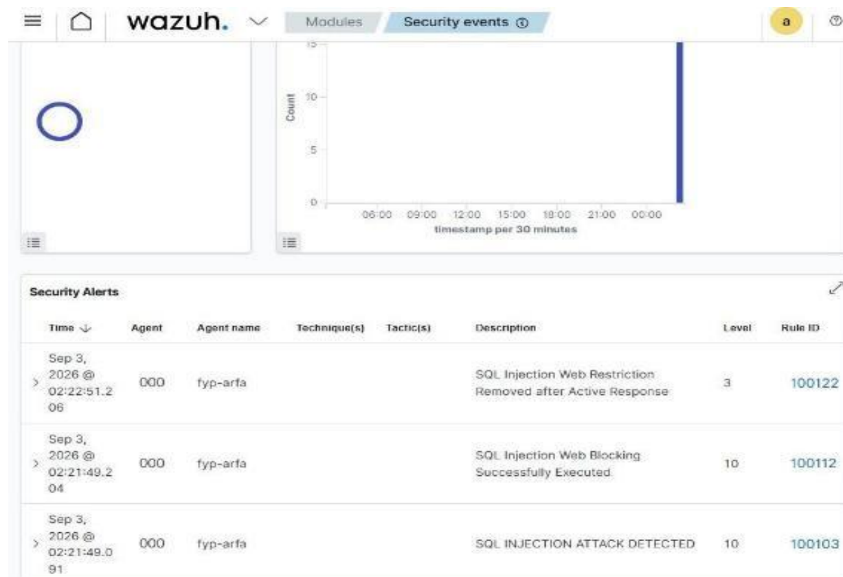
Figure 9. Wazuh sequence for SQL-injection detection, temporary blocking, and response removal.
