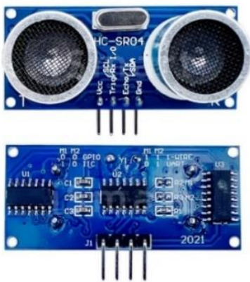
Fig. 2 Ultrasonic sensor HC-SR04
