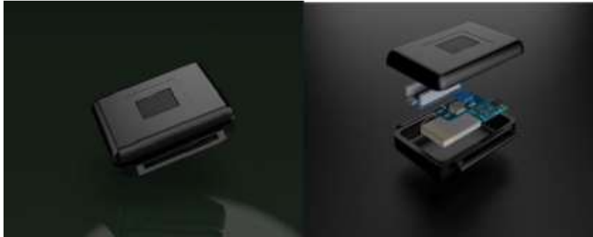
Figure 2.1 3D View of the Bracelet Enclosure Design
