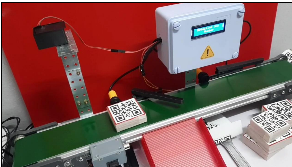
Figure 1 - ESP32-CAM-based QR code recognition system showing overall system architecture.
