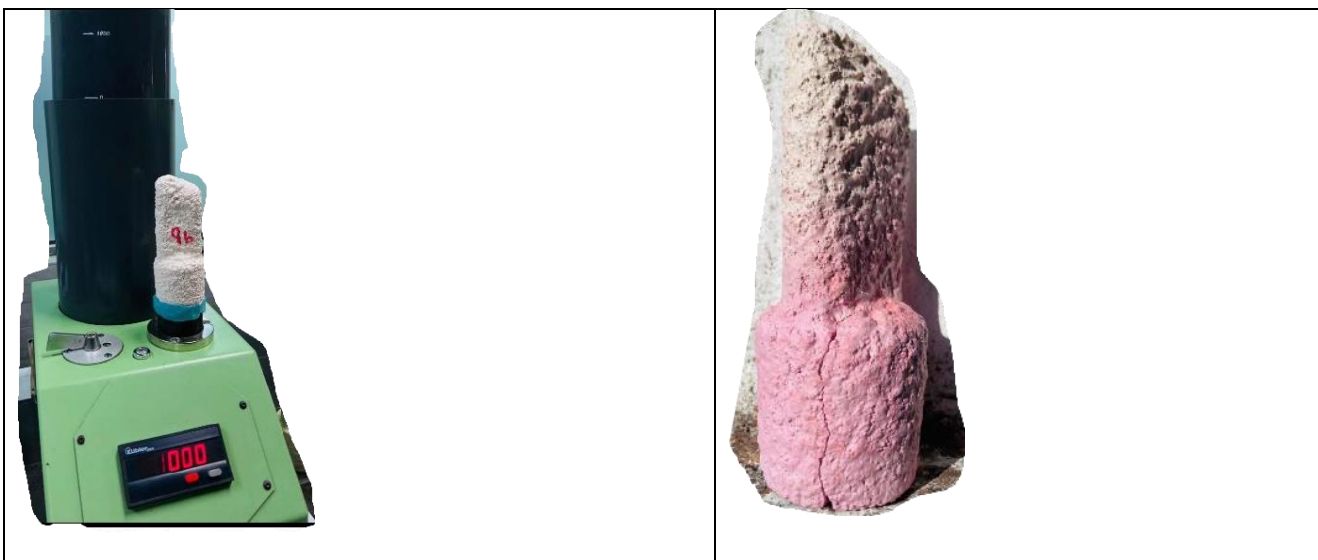
Figure 1. Air Permeability Test & Dye Penetration Test (NDT) Sample
