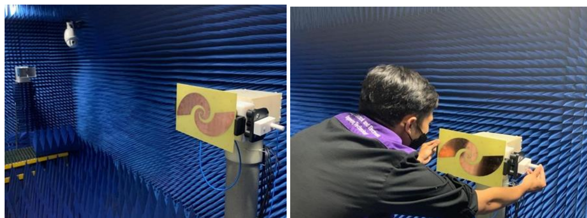
Figure 6. Anechoic Chamber and Measurement Setup
