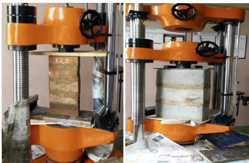
Fig. 7 Test setup of brick masonry prism and solid concrete block masonry prism
