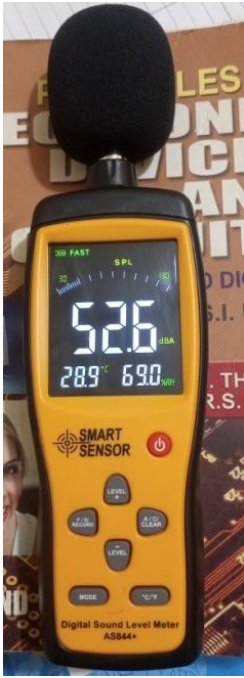
Figure II: Digital Sound Level Meter AS844+ (Source: Physics Laboratory, Lagos State University of Science and Technology).
