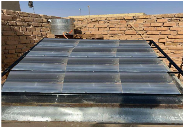
Fig (1) Solar still with Fresnel lenses
