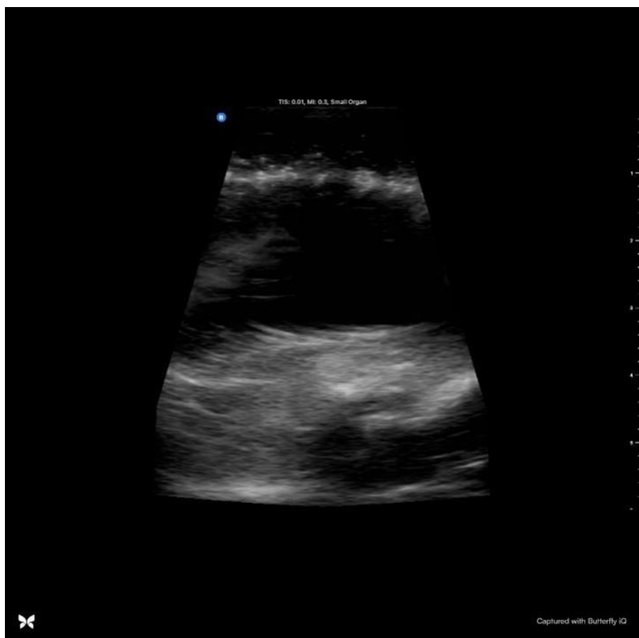
Figure 3 Cancerous lesion seen in the breast phantom tissue using point of care ultrasonic device
