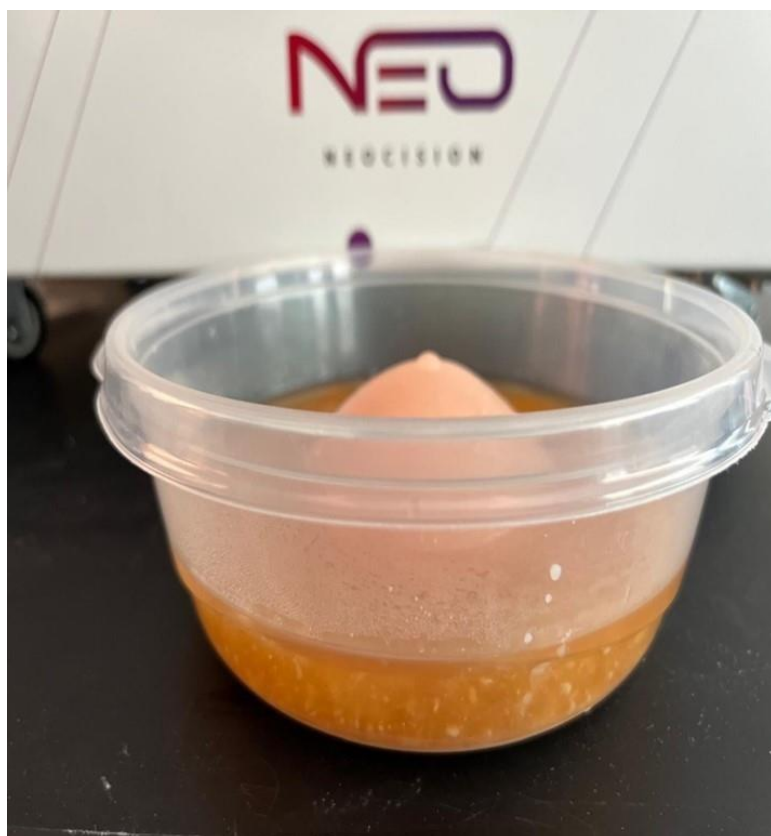
Figure 5 Phantom breast tissue created from tissue mimicking materials in the lab
