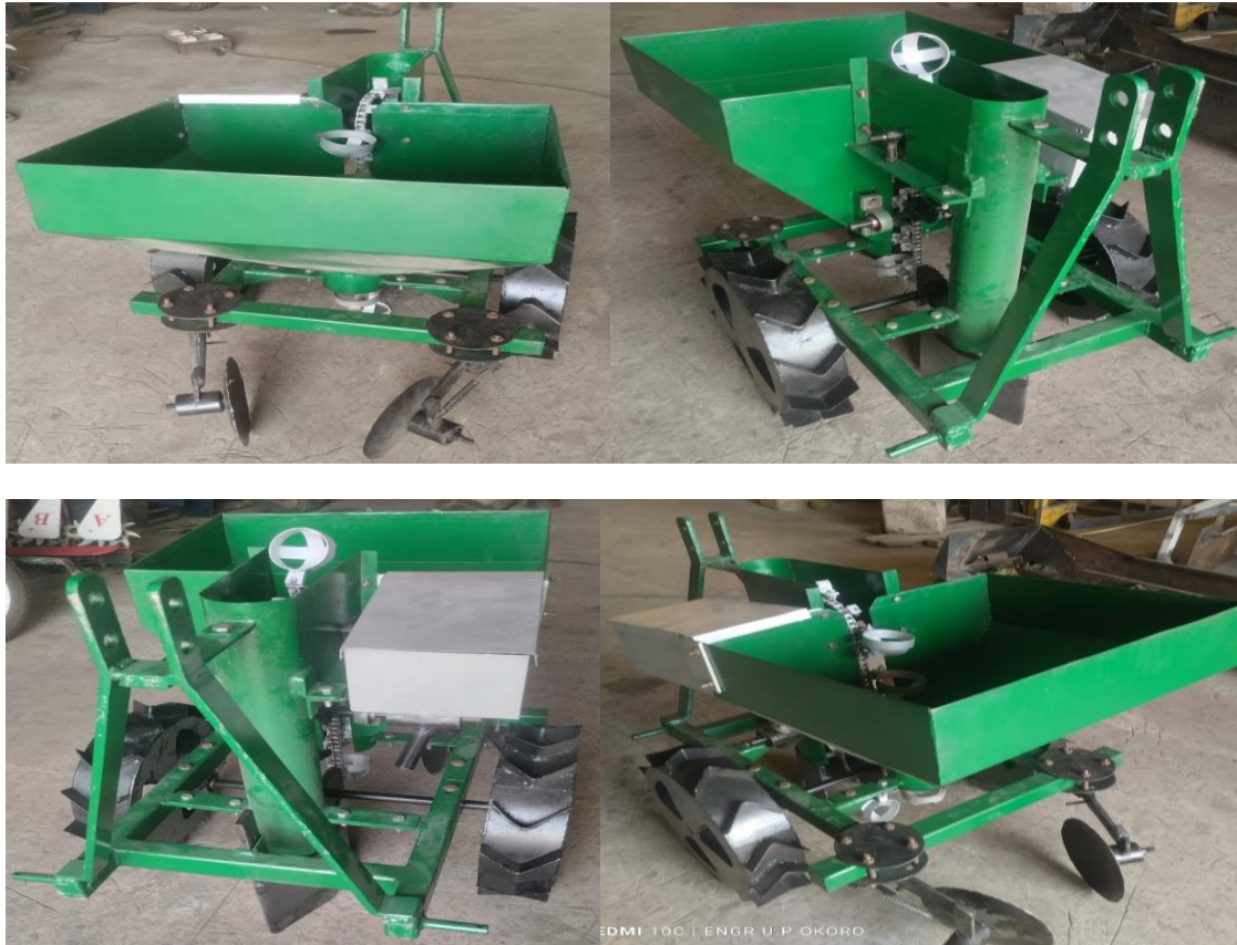
Plate 3.1: Pictorial view of the developed tractor-drawn single row Irish potato planter with fertilizer applicator.
