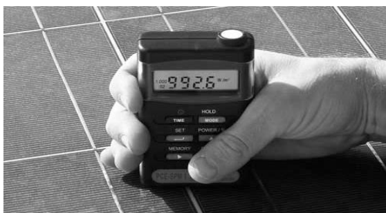
Fig. 1. Traditional way of Solar radiation measurement.
