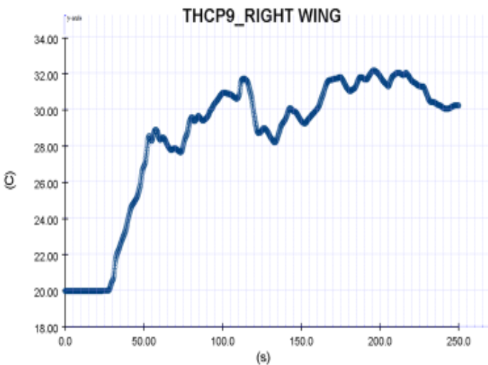
Figure 9 (i): Thermocouple 9 at 29.5m above the 9 th floor.
