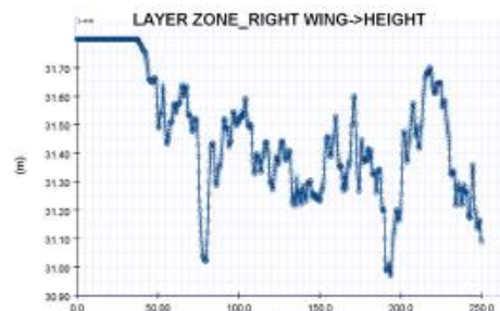
Figure 7(d): Right Wing Smoke Layer Height
