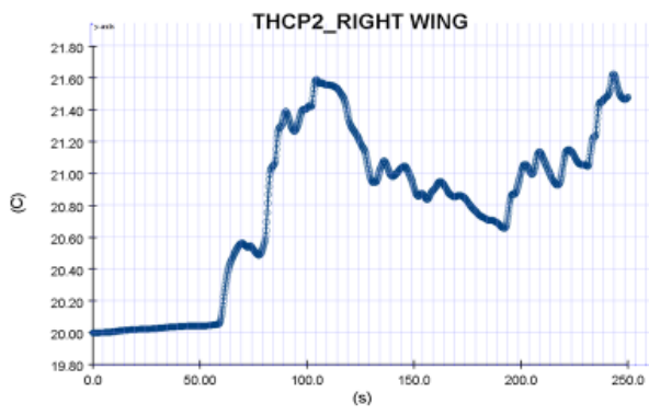
Figure 9 (b): Thermocouple 2 at 9.7m above the 2 nd floor.
