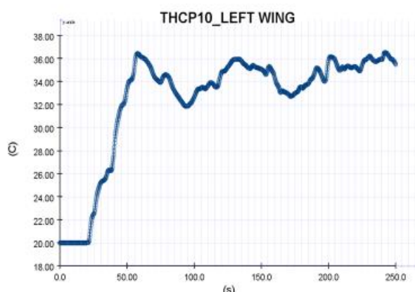
Figure 8 (j): Thermocouple 10 at 29.5m above the 9 th floor.
