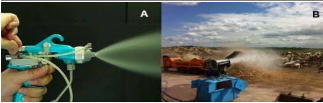
Fig. 11: A=Spray gun. B=Dry fog application. A and B are examples of dust suppression technologies used to reduce dust particles in the quarry site (Garcia-Granda et al., 2024)
