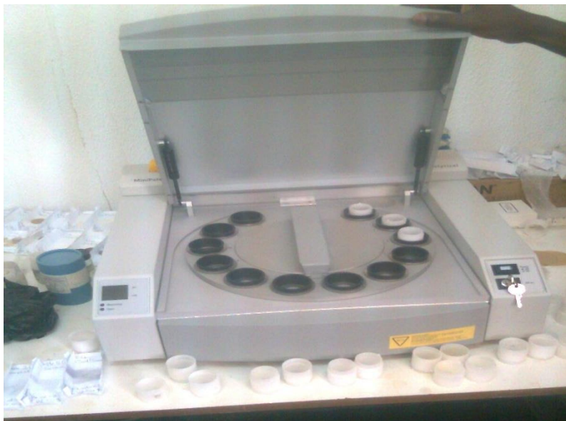
Figure 4: The Mini pal 4 Spectrometer with Displayed Pellets
