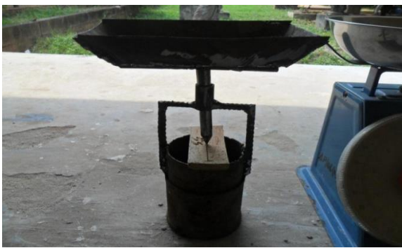
Figure 5: Locally fabricated Modulus of Rupture Machine
