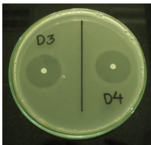
Figure 12: Photographic representation of zone of inhibition of NPs Chi-Cu(II) and Chi-Cd respectively against the bacteria Escherichia coli .
