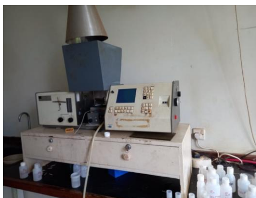
Figure 3: Atomic Absorption Spectrometry instrument used for analysis.
