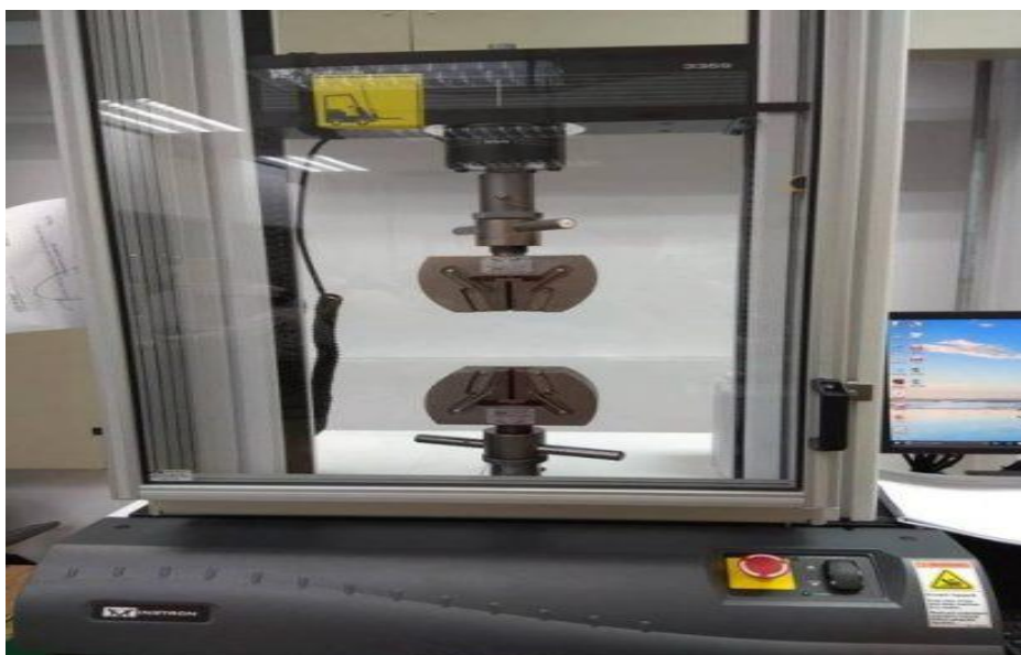
Plate 2: Tensile Strength of UTWHF Using Universal Instron Testing Machine
