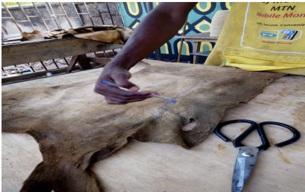
PLATE 1. 6: The template was traced and cut out from the dry leather which will serve as reinforcement. Three layers were cut out.
