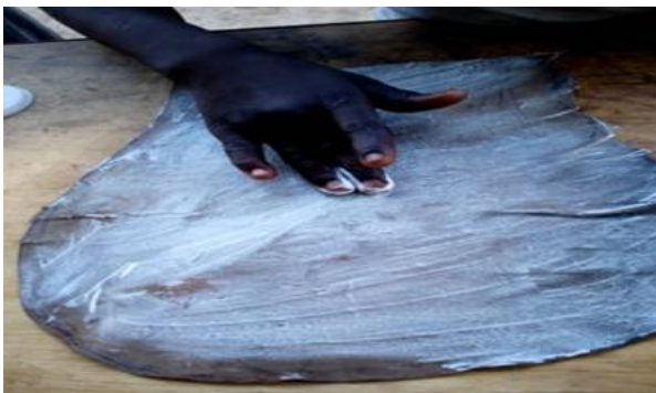
PLATE 1.7: white glue was applied to the grain side of the cut-out templates for moulding.
