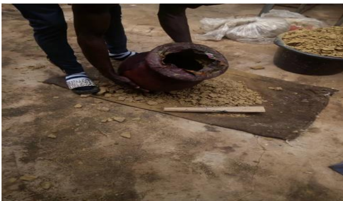
PLATE 1.12: Clay pot is the broken and clay is pour away leaving the moulded leather.
