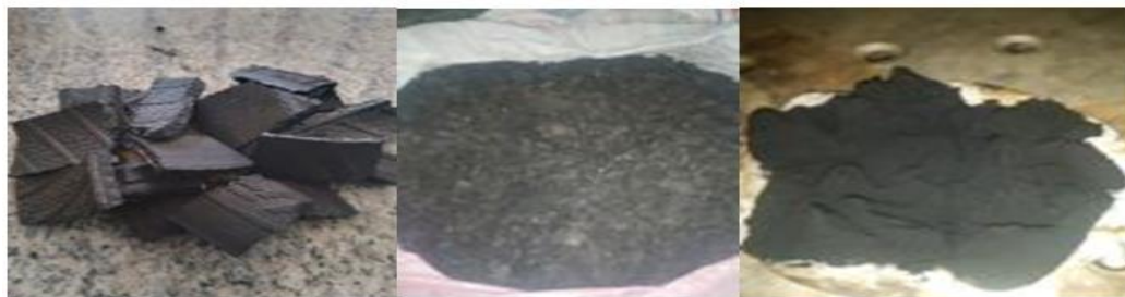
Figure 2a, b & c: Shredded pieces of tire before, pyrolysis image of sample after pyrolysis and dried pigment sample after demineralization
