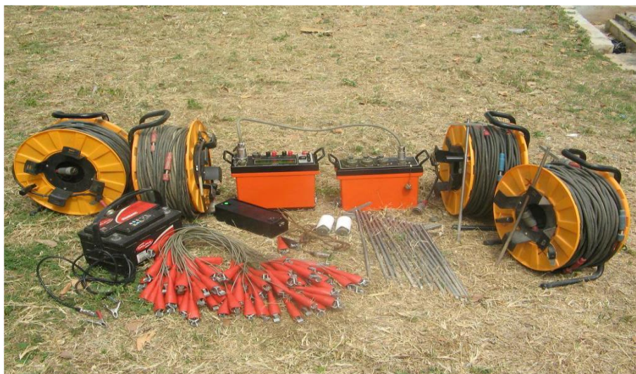
Plate 2: ABEM LUND Imaging System together with Terrameter SAS 1000 and ES 464 used for Electrical Resistivity Tomography
