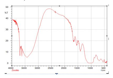
Fourier Transform Infrared (FTIR) Spectrometer showed characteristic peaks of both zeolite and magnesium-sulfate load with zeolite. Key absorptions included
