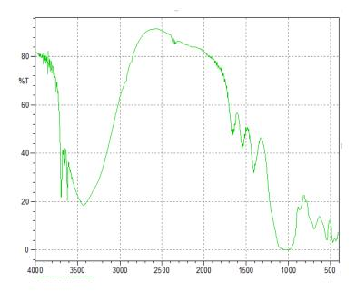
Symmetric stretching of T–O–T (T = Si or Al), Double ring or cage vibrations, characteristic of zeolite structure.
