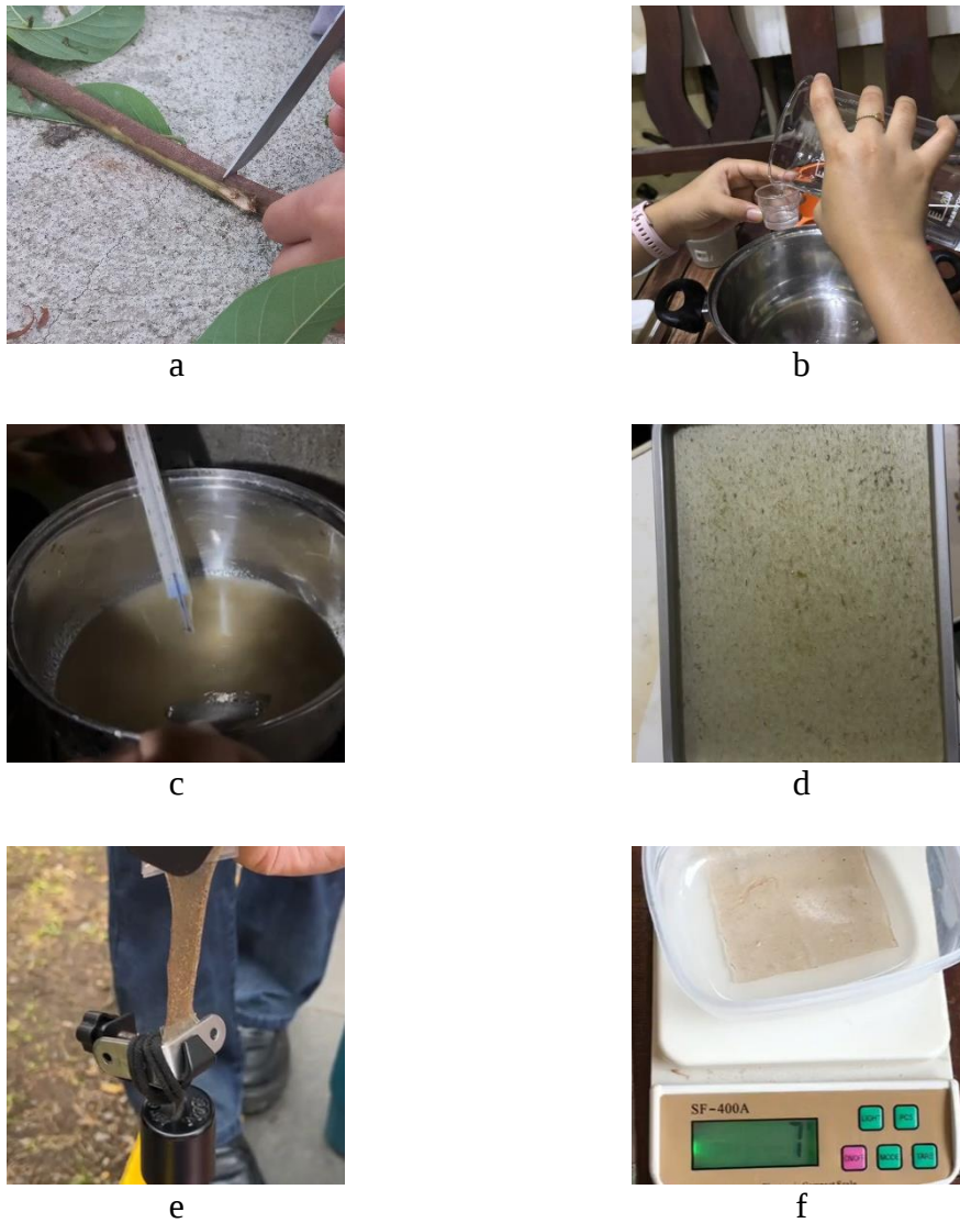
Figure 1. Production of bioplastic. (a) Preparation of atis fiber; (b) Formulation of bioplastic base solution; (c) Mixing the formulation of atis fiber mixture; (d) Molding of atis fiber mixture; (e) Performance assessment for tensile strength test; (f) Performance assessment for water absorption.
