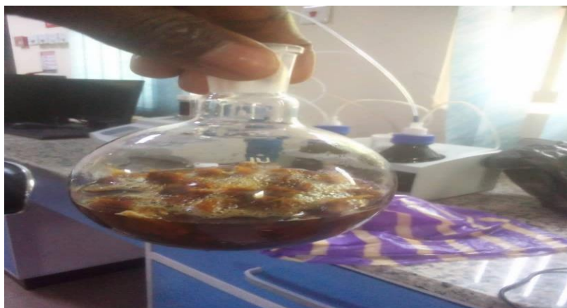
Figure 2.2 Mixture of Bamboo and NaOH solution after heating
