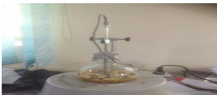
Figure 2.1 Mixture of Bamboo and NaOH solution before heating
