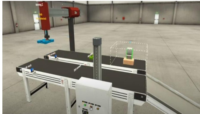
Figure 6: Simulation of final inspection in Factory IO
