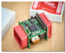
The Main Controller (MC) is the brain of the system, it communicates with all ESCs and RC transmitter to carry out the autopilot functionality. It has a built-in Inertial Measurement Unit (IMU) consists of one 3-axis accelerometer, one 3-axis gyroscope and a barometer for sensing the attitude and altitude.
