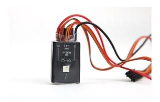
Specially designed for NAZA-M LITE. It solves the high power consumption problem of multi-rotor system, supply and monitor power for NAZA-M LITE and other electronic devices. It also has an LED to indicate different operating states of NAZA-M LITE and a USB interface for configuring the NAZA-M LITE unit and firmware upgrade.
